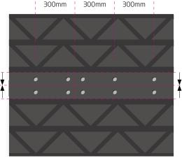
Place joining strip with half sticking out from the edge
